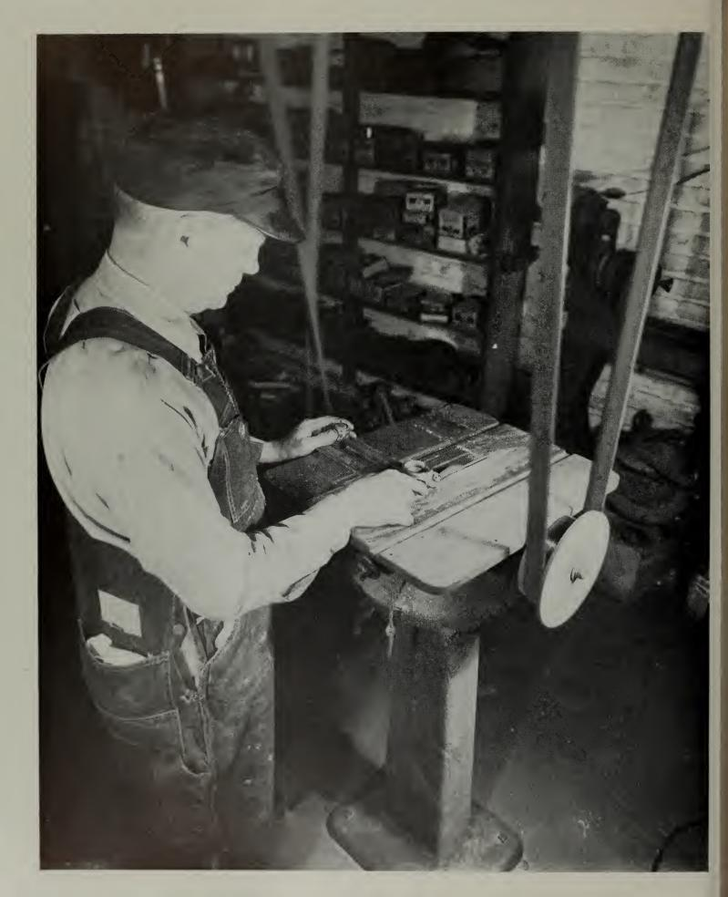
The Model  $\Lambda$  connecting rods are now on a saw table in which a rotating saw blade cuts the babbitt flange to complete the separating operation as shown in Picture 24. This also cuts the necessary oil relief groove through the flange.
